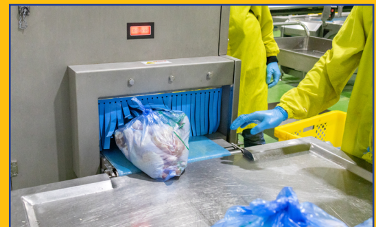
→ Chicken meat passing through an X-ray inspection machine.
