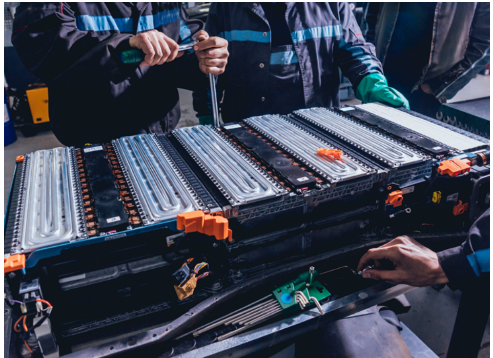
Disassembling the battery of an electric vehicle.
