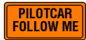
Traffic needs to follow this vehicle to get safely through the work zone.
